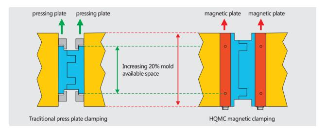
During Production Processing, too much time is wasting due to the mechanical clamp selection. Owing to magnetic quick mold change system uniform clamping mold back space, avoid mechanical fake clamping and other dangerous circumstance happen.
